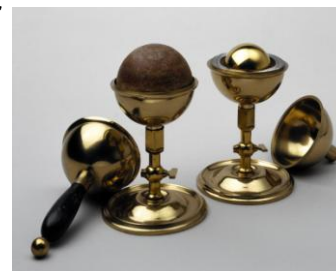
Fig. 10.1: Spherical capacitors used by Faraday. Faraday showed that when dielectric material was placed between the central brass ball and a concentric brass shell, the capacitance of the spherical capacitor increased manifold. The factor by which it increased was different for different dielectric materials. (Source:
