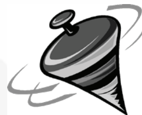
Fig. 11.2: When an object rotates about an axis passing through it, all points on the object move in a circle. The centres of the circles lie on a straight line that is called the axis of rotation.
