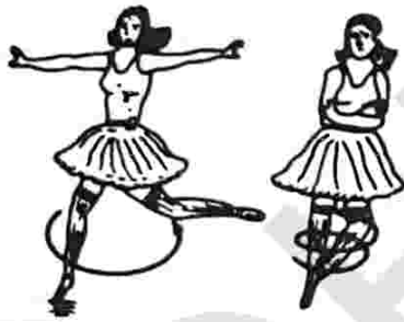
Fig. 7.67 A ballet dancer increases \omega by changing to a posture of smaller M.I.
