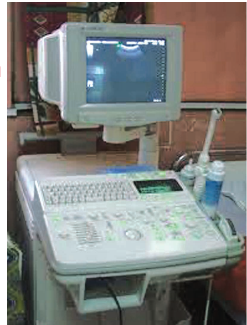
Figure 48. This is an ultrasound machine which is used in hospitals. It produces ultrasound scans of the inner organs of human body such as liver, gall bladder, pancreas, kidneys, uterus and heart, etc.
