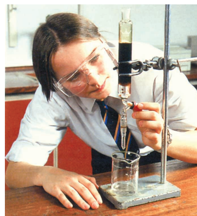
Figure 70. The separation of two (or more) immiscible liquids by a separating funnel is based on the difference in their densities. In this photograph, a student is separating a mixture of water and oil by using a separating funnel. Water is denser than oil so it sinks to the bottom of separating funnel. When the tap is opened, the water can be run off first.
