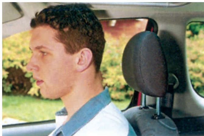
Figure 16. This photograph shows a 'head restrain' at the back of person's neck sitting in a car. Head restrains are provided in cars to reduce neck injury in case of an accident. They are particularly effective in rear-impact accidents (when a vehicle hits from behind). Can you describe how ?
