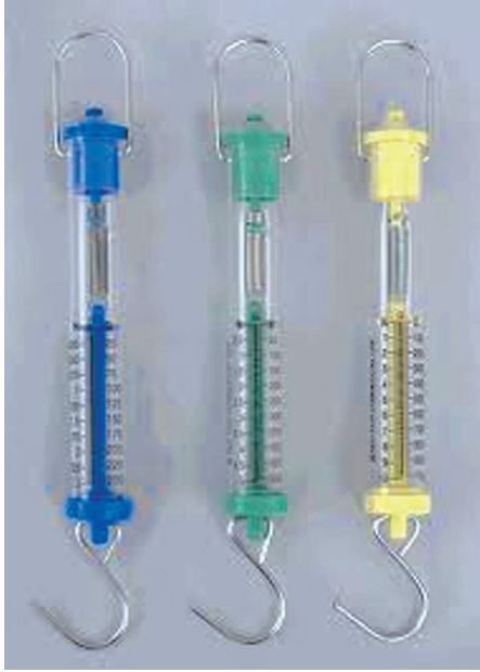
Figure 35. These are spring balances. They are used to measure weight of objects.
