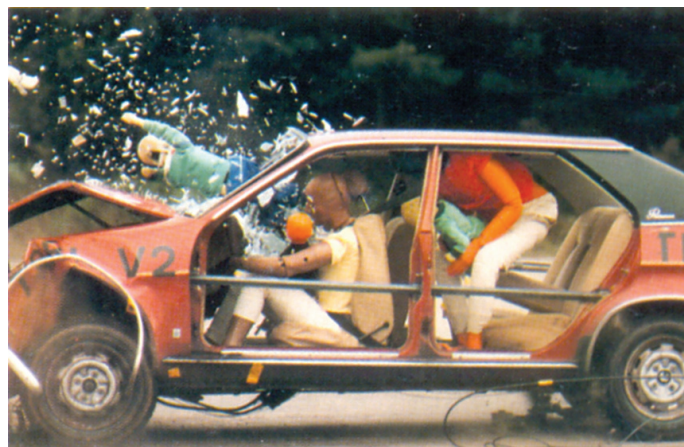
Figure 23. This is what can happen if passengers do not wear seat belts while travelling in a car and the car stops suddenly due to an accident. The large force on the body of passengers produced by rapid decrease in momentum can throw the passengers forward violently causing serious injuries.
