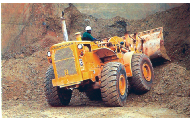
Figure 49. The wide tyres of this tractor spread the weight of tractor and its trolley over a large area of ground producing lesser pressure on ground so that it can travel over soft or muddy ground without sinking in it.
