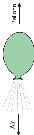
Figure 36. A deflating balloon also demonstrates the principle of working of a rocket.
