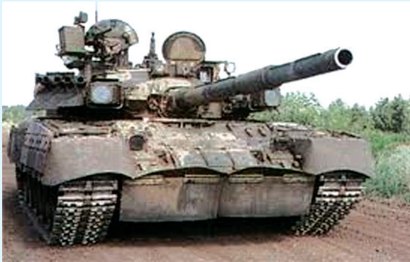
A wide steel belt is provided over the wheels of an army tank.
