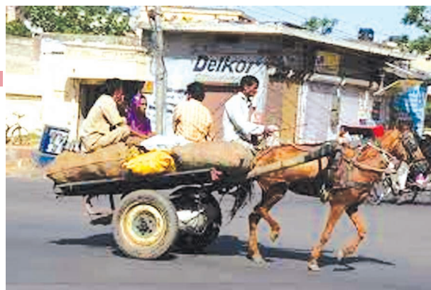
Figure 40. To make the cart move, the horse bends forward and presses the ground with its feet. When the forward reaction to the backward push of the horse is greater than the opposing frictional forces of the wheels, the cart moves.
