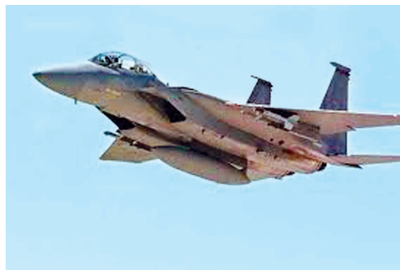
Figure 33. This jet aircraft flies at supersonic speed. Its speed (2650 km/h) is more than twice the speed of sound (which is about 1200 km/h). This jet aircraft produces sonic boom in the area where it flies.
