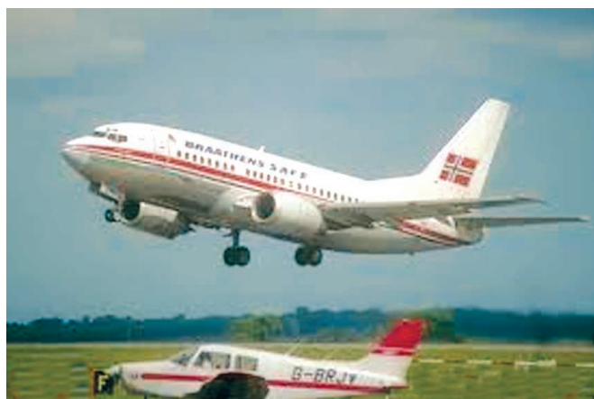
Figure 69. Aluminium is a light metal having comparatively low density. Aircraft is made from aluminium alloys to give it a low density (to keep it light), and high strength.
