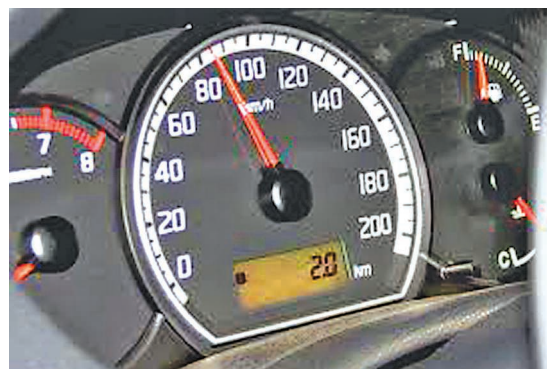
Figure 11. Speedometer and odometer of a car. This speedometer shows a speed of 85 km/h and odometer shows a reading of 2.0 km for the distance travelled by the car so far. The distance travelled suggests that it is a brand new car.
