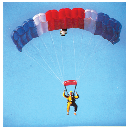
Figure 25. Due to its special design to make air resistance as large as possible, a parachute decelerates as it falls towards the ground. It has a negative acceleration. By using parachute, this man will land on the ground safely with a speed of only about 8 m/s.
