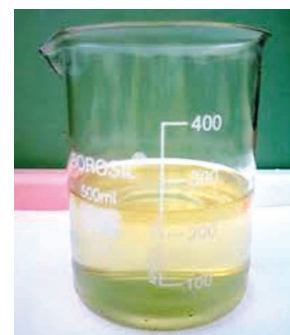
(c) The density of glycerine is higher than that of water. So, glycerine will exert more buoyant force on an object immersed in it (than water)
