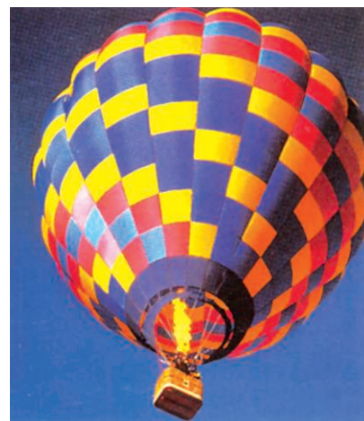
Figure 58. It is the buoyant force (or upthrust) due to displaced air which makes this hot-air balloon rise up in the air.
