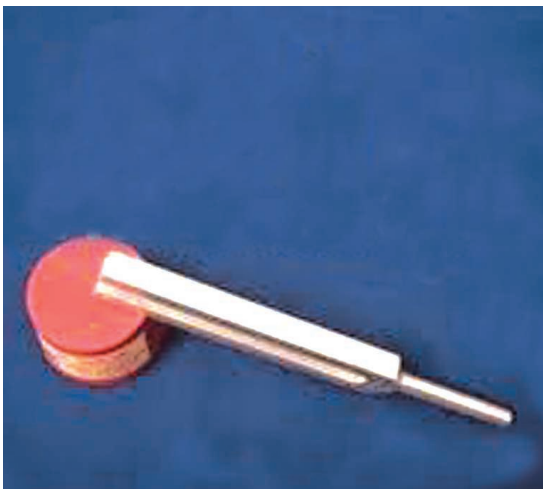
Figure 20. This photograph shows a tuning fork along with the hard rubber pad on which it is struck to produce sound.
