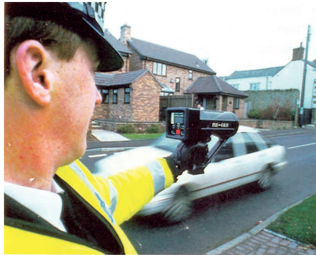
Figure 14. This photograph shows a traffic police officer using the speed gun (or radar gun) to determine a running car's speed. The overspeeding drivers are fined heavily.
