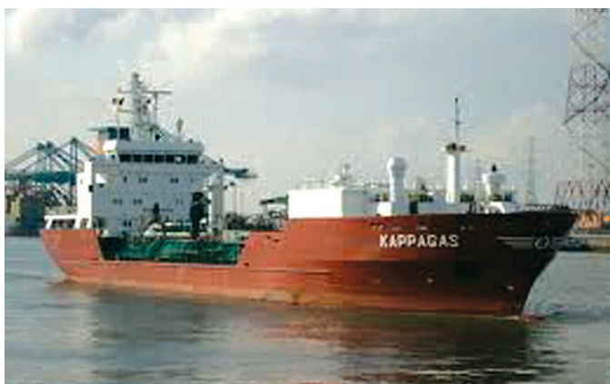
Figure 66. A ship floating in water. When the ship is inside the sea, it sinks in the sea water to a certain level such that the weight of sea water displaced by its submerged part is equal to the whole weight of the ship.
