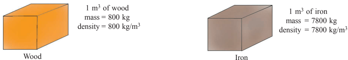
Figure 68. The mass of 1 cubic metre volume ( 1 \text{ m}^3 ) of a substance is known as its density.
