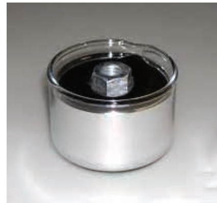
(c) Iron floats in mercury because the density of iron is less than that of mercury
