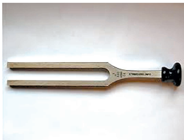
Figure 26. This is a tuning fork of frequency 256 Hz. When the prong of this tuning fork is struck on a hard rubber pad, it will vibrate with a frequency of 256 Hz and produce sound waves of frequency 256 Hz.
