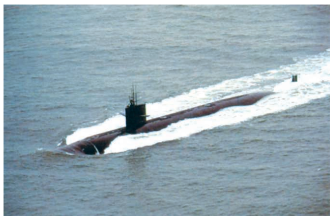
Figure 67. A submarine sinks in the sea by taking water into its buoyancy tanks (so as to increase its weight). Submarine can again come to the surface of sea by blowing water out of its buoyancy tanks by using compressed air (so as to reduce its weight).
