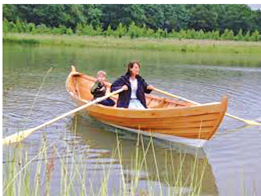
Figure 38. The woman pushes the water backwards with the oars. The backward going water exerts an equal and opposite push on the boat (which makes the boat move forward).
