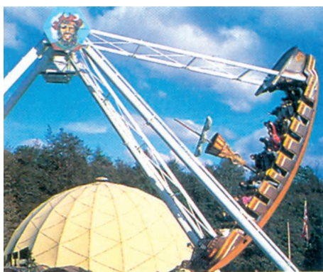
Figure 48. In this fun-fair ride called 'Pirate Ship', kinetic energy is changed into potential energy and back into kinetic energy (as in a simple pendulum).
