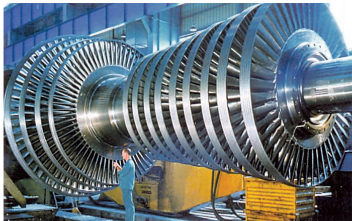
Figure 53. This is the steam-turbine assembly for a thermal power house generator. We can see the large number of turbine blades in this photograph. The superheated, high pressure steam is used to turn this turbine which is connected to the electric generator for producing electricity. All of us should save on electricity so as to conserve our precious fossil fuels like coal and natural gas.
