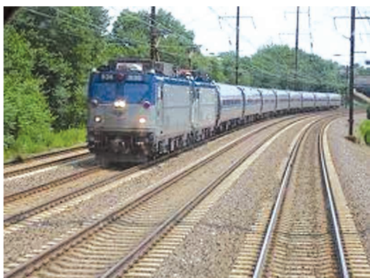
Figure 41. This electric train engine can provide 2 megawatts (2 MW) of power to drive the train at full speed. This power is more than 2680 b.h.p.
