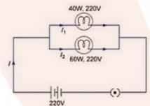
(b) Voltage across both the bulbs is same and is equal to 220V. Current through 40W lamp =  $I_1 = P_1/V = 40/220 \text{ A}$ Current through 60W lamp = I2 = P2/V = 60/220 ATotal current drawn from the electric supply = 40/220 + 60/220 = 0.45 A
