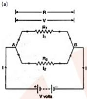
Suppose total current flowing the circuit is I, then the current passing through resistance R<sub>1</sub> will be I<sub>1</sub> and current passing through resistance R<sub>2</sub> will be I<sub>2</sub>.
