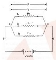
Suppose total current flowing in the circuit is I, then the current passing through resistance R<sub>1</sub> will be I<sub>1</sub>, current passing through resistance R<sub>2</sub> will be I<sub>2</sub> and current passing through resistance R<sub>3</sub> will be I<sub>3</sub>.
