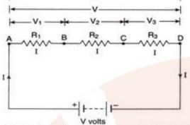
(a) Fig shows three resistances R<sub>1</sub>, R<sub>2</sub> and R<sub>3</sub> connected in series with a battery of V volts. Let the p.d. across R<sub>1</sub>, R<sub>2</sub> and R<sub>3</sub> is V<sub>1</sub>, V<sub>2</sub> and V<sub>3</sub> respectively.
