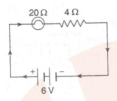
(a) Total resistance of the circuit=R<sub>1</sub>+R<sub>2</sub>=20+4=24ohm
