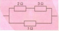
Resistance of first line = 2+3 = 5 ohm So, 1/R = 1/5 + 1/5 On solving we get that R=2.5ohms
