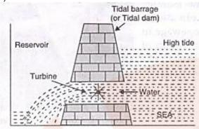
(a) At high tide, water flows from sea into reservoir and turns the turbine
