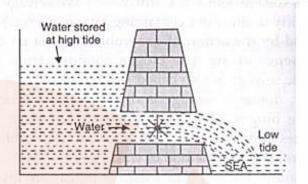
(b) At low tide, stored water flows out from reservoir into sea and turns the turbine
