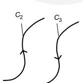
Fig. 3.10: The line integral over the path  $C_2$  will be the negative of the line integral over the path  $C_3$  $\int \vec{F}.d\vec{I} = - \int \vec{F}.d\vec{I}$  $C_2 \qquad C_3$
