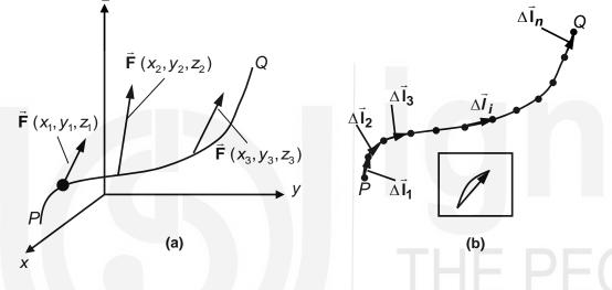
Fig. 3.3: a) An object moves under a variable force along the path *PQ*. The force is different at different points along the path; b) the path is divided into *n* segments and the displacement is defined for each segment.
