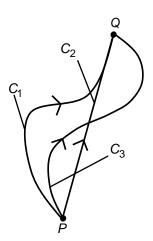
Fig. 3.11: Three different paths of integration between two points Pand Q,  $C_1$ ,  $C_2$  and  $C_3$ . If the line integral of a vector field  $\vec{F}$  has the same value for all these paths then  $\vec{F}$  is a conservative vector field.
