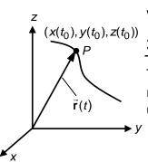
Fig. 3.5: Parametric representation of a curve. At the point *P*, the value of the parameter is  $t_0$ , the position vector is  $\vec{r}(t_0)$  and the coordinates are  $(x(t_0), y(t_0), z(t_0))$ .
