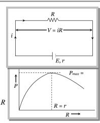
(vii) **Short trick to calculate** E **and** r: In the closed circuit of a cell having emf E and internal resistance r. If external resistance changes from  $R_1$  to  $R_2$  then current changes from  $i_1$  to  $i_2$  and potential difference changes from  $V_1$  to  $V_2$ . By using following relations we can find the value of E and r.
