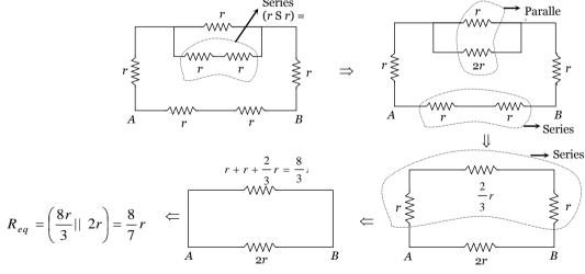
**Example: 39** In the given figure, equivalent resistance between A and B will be
