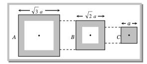
Solution: (a) All the conductors have equal lengths. Area of cross-section of A is  $\{(\sqrt{3} \ a)^2 - (\sqrt{2} \ a)^2\} = a^2$
