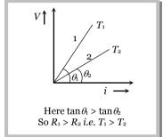
(2) The device or substances which doesn't obey ohm's law *e.g.* gases, crystal rectifiers, thermoionic valve, transistors etc. are known as non-ohmic or non-linear conductors. For these *V-i* curve is not linear. In these situation the ratio between voltage and current at a particular voltage is known as static resistance. While the rate of change of voltage to change in current is known as dynamic resistance.
