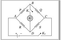
(ii) **Unbalanced bridge**: If the bridge is not balanced current will flow from *D* to *B* if  $V_D > V_B$  i.e.  $(V_A - V_D) < (V_A - V_B)$  which gives PS > RQ.
