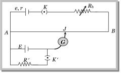
(2) Comparison of emf's of two cell: Let  $l_1$  and  $l_2$  be the balancing lengths with the cells  $E_1$  and  $E_2$ respectively then  $E_1 = xl_1$  and  $E_2 = xl_2 \implies \frac{E_1}{E_2} = \frac{l_1}{l_2}$
