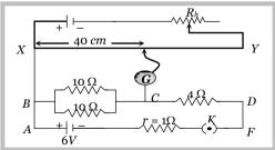
Solution: (a)  $\frac{1}{R} = \frac{1}{10} + \frac{1}{10} = \frac{2}{10} = \frac{1}{5} \text{ or } R_1 = 5 \Omega$
