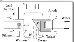
The filament is heated by pass applied between the target and cath highly energetic electrons are focus window W is W indow W in W in
