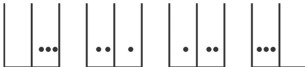
Figure A.1 Example of possible distributions of three particles between two states.
