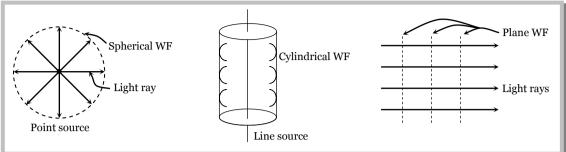
(v) Every point on the given wave front acts as a source of new disturbance called secondary wavelets. Which travel in all directions with the velocity of light in the medium.
