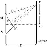
and For minima at  $P: \quad \Delta = \frac{(2n-1)\lambda}{2}$ ; where  $n = \pm 1, \pm 2, \dots$
